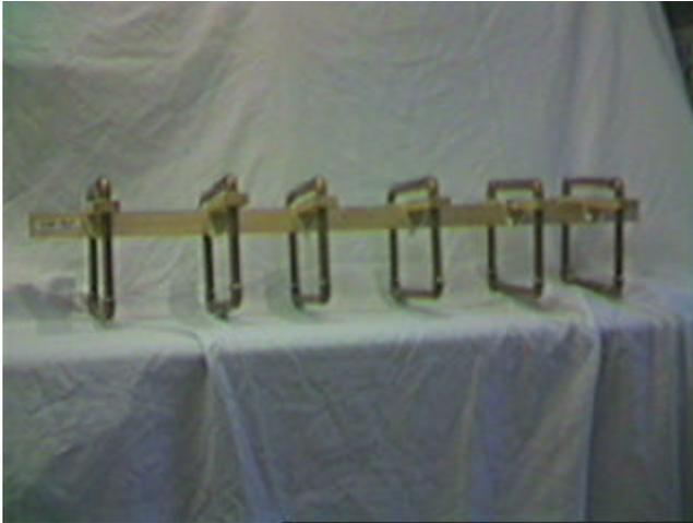
Figure 3 - KF8QU "copper pipe" attic antenna
