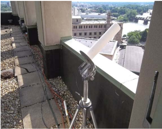
The antenna on the left receives the camera video from the AEP roof. The photo on the right shows our control station with 2 split screen monitors to view the data inside the mezzanine on the Police building 12 th floor. To its right is the 1270MHz receivers for the AEP video and camera control.
