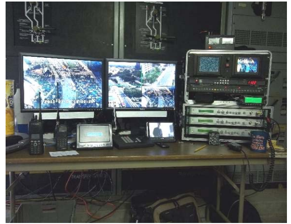
The antenna on the left receives the camera video from the AEP roof. The photo on the right shows our control station with 2 split screen monitors to view the data inside the mezzanine on the Police building 12 th floor. To its right is the 1270MHz receivers for the AEP video and camera control.
